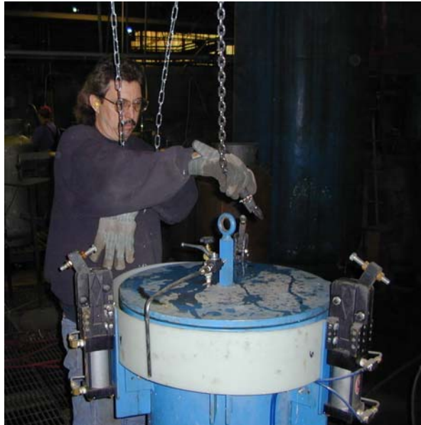
Figure A-3. Water jacket lid and chain hoist used for lifting and lowering
