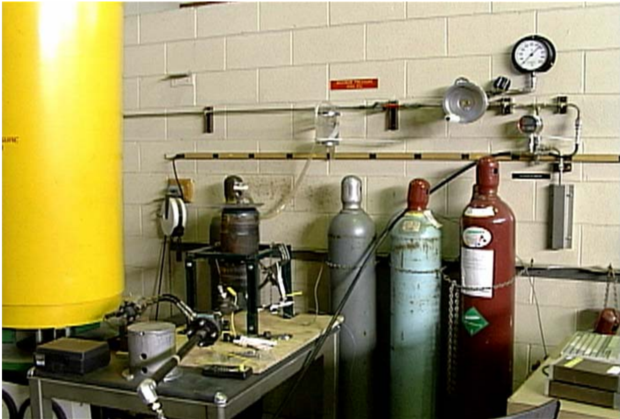
Figure A-9. Apparatus and equipment used to test relief valve performance.
