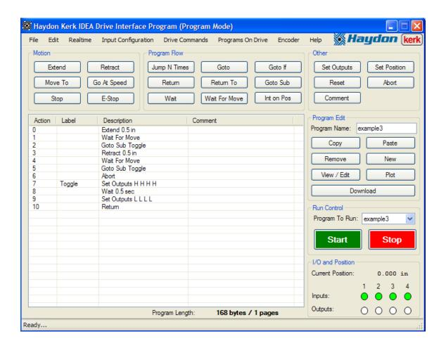
**Example Four:** This example is different in that the actuator does not need to start in the fully retracted position. We will perform a homing routine, to find the fully retracted position, and then move to 0.5" from that point, wait 1 second, and then return to the fully retracted position.
