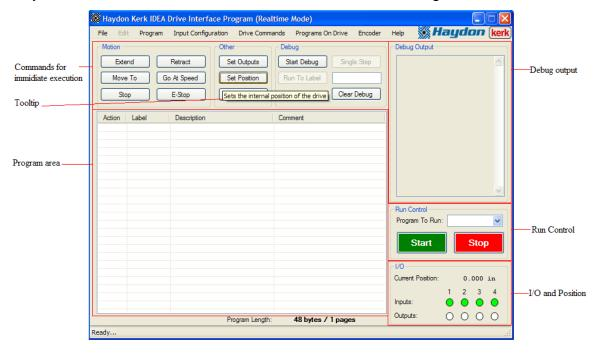
In the Realtime mode, each command executed from the "Commands for immediate execution" section elicits an immediate action from the drive.
