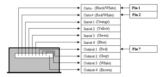
Open Collector Output Pin Diagram
