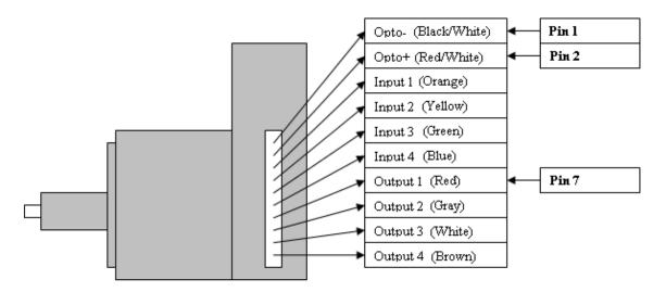
Stand alone drive I/O connector, pin identification:
