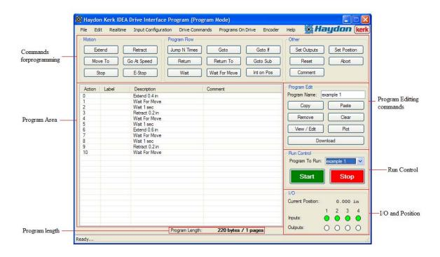
The I/O and position section provides constant feedback from the drive pertaining to the current state of the drive. This area can also be used to control the state of the outputs, as well as the inputs if in simulation mode.
