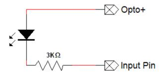
The IDEA drive has four optically isolated inputs and four optically isolated open-collector outputs. The voltage range for these is 5-24VDC. As the outputs are open-collector, they will need a pull-up resistor tied to the Opto-supply. The outputs are capable of sinking up to 200mA each.
