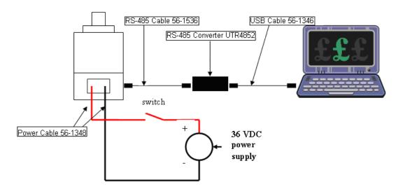
• After wiring as shown, turn on power supply and close the switch.
