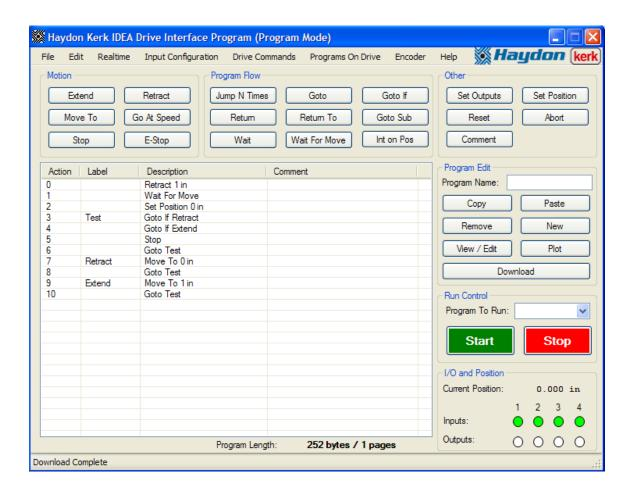
**Example Six:** In this example, we will first find the fully retracted position of the actuator. The actuator will continuously move in the extend direction, until getting 0.9" from the fully retracted position. When the 0.9" position is reached, the actuator will retract back to the 0" position, and resume the extend. If at any time during the program, input 1 changes state, the program will abort.
