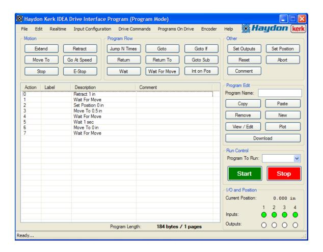
**Example Five:** In this example, we will first find the fully retracted position of the actuator, then the actuator will move to the 0" position if input 1 is high and input 2 is low, move to the 1" position if input 1 is low and input 2 is high, or stop if inputs 1 and 2 are both high, or both low.
